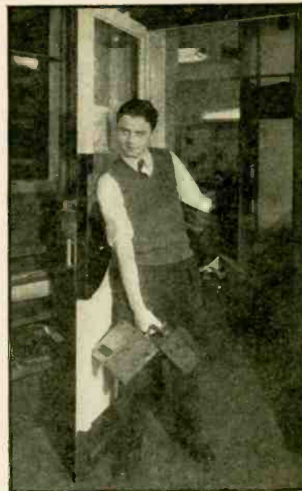
Fig. 3.—How NOT to carry valuable instruments. Meters are easily injured. They deserve attentive and very careful handling.
