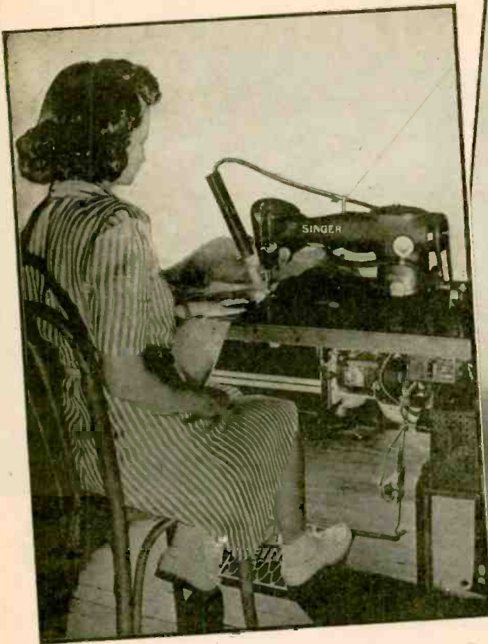
Left: a standard machine fitted with the electronic guard. Right, a closer view of the details of the "seeing-eye" device.
